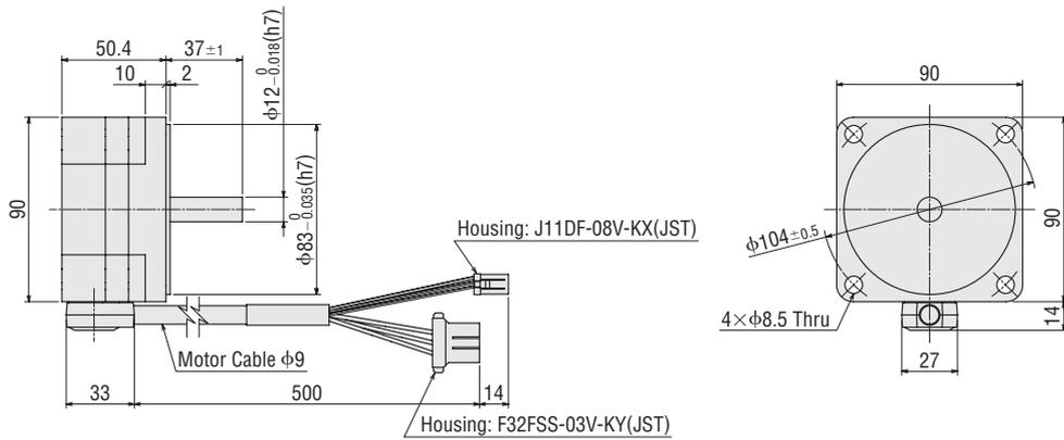
• Cable output in the opposite side of the output shaft
