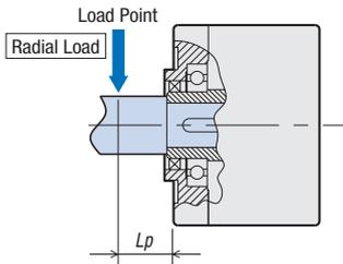
$F_0$  [N] : Permissible radial load on flange-installation surface
