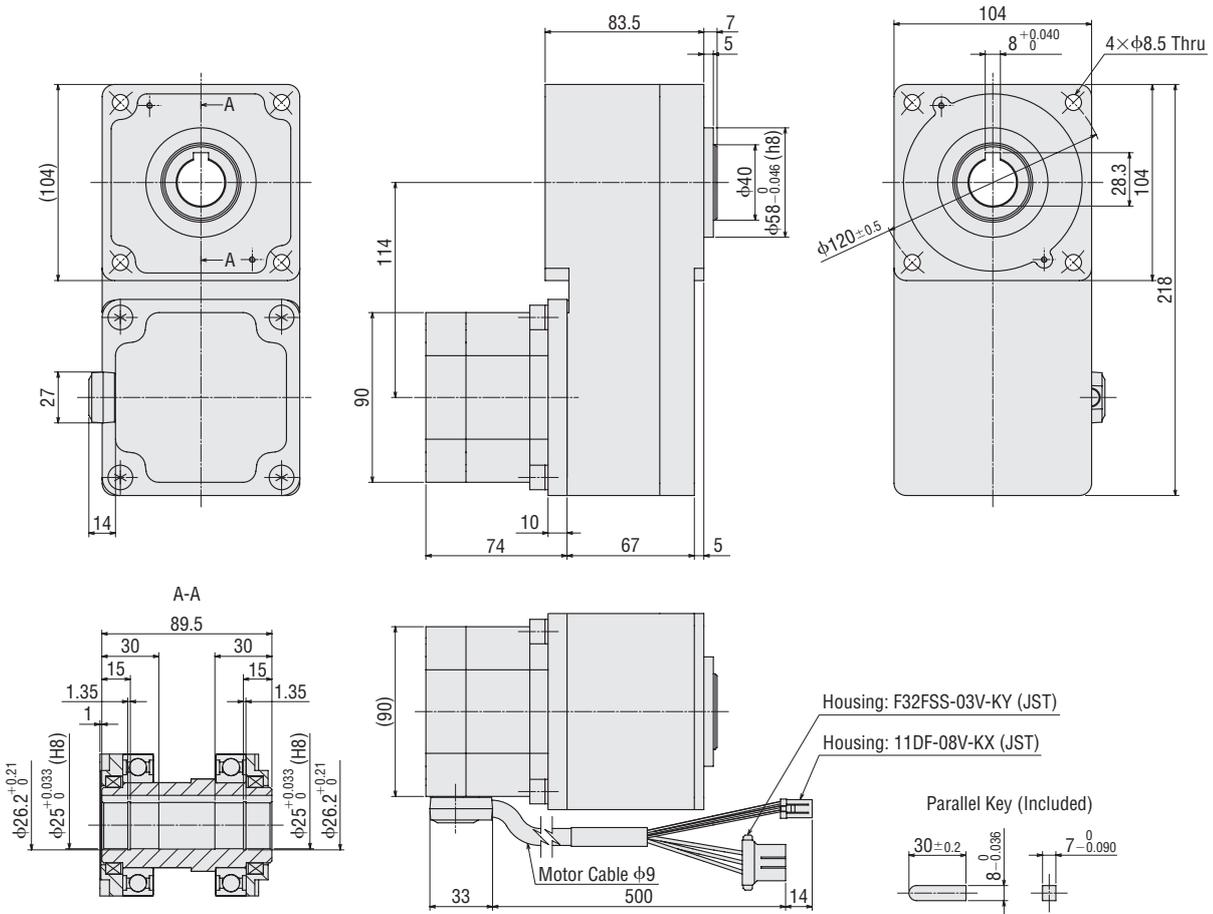
• Cable output in the opposite side of the output shaft
