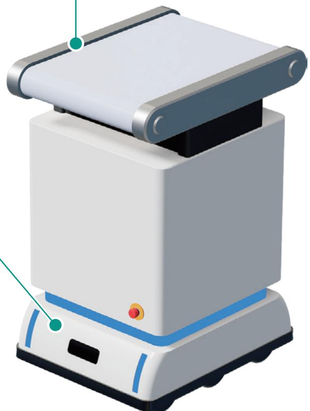
Application: Autonomous transportation robot with belt conveyor
