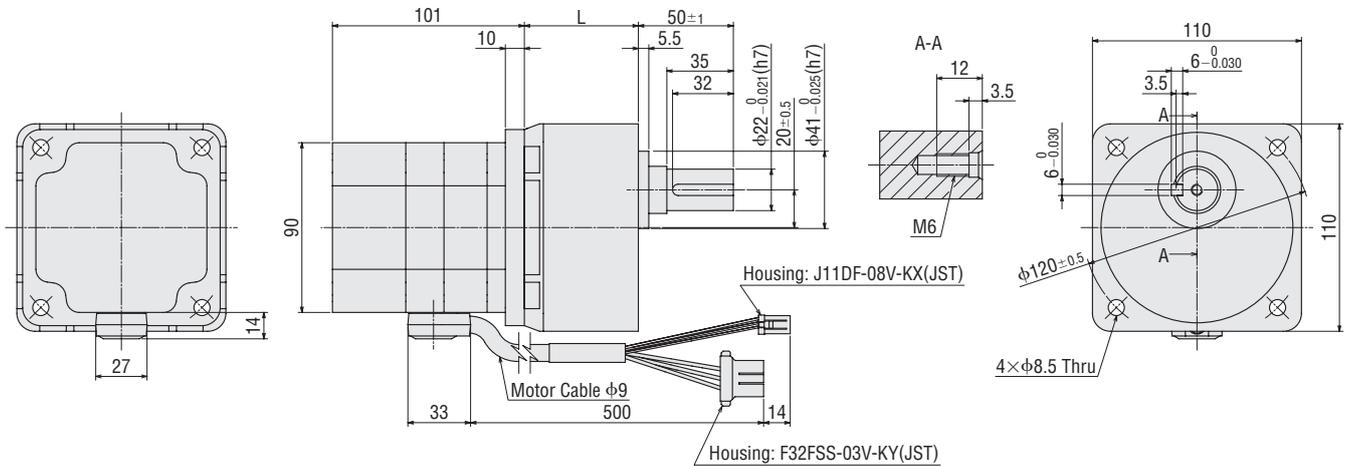
● Cable output in the opposite side of the output shaft
