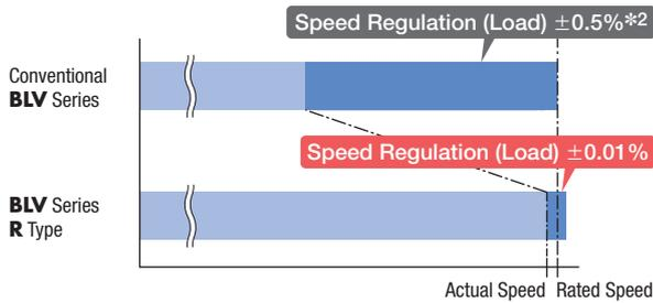
\*1 Rate of change in speed when a constant load is applied
