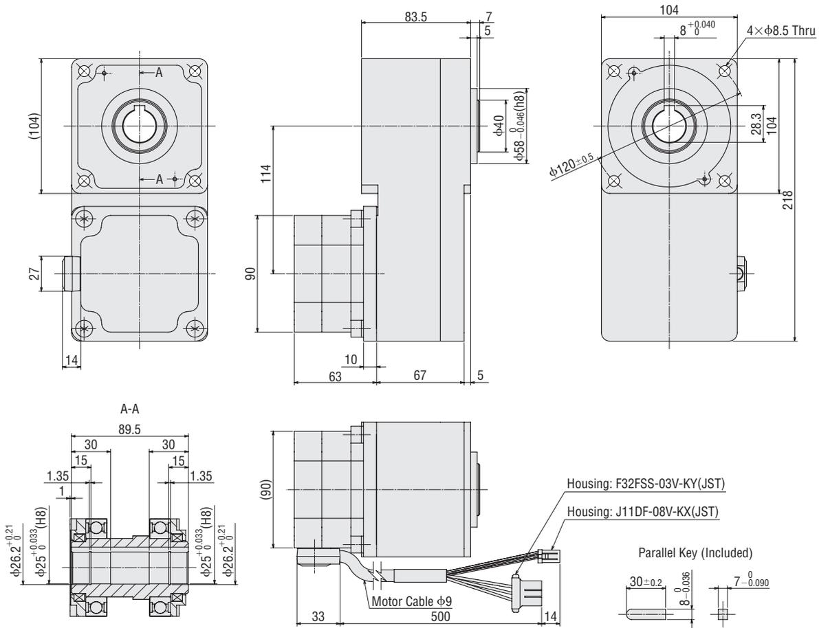
• Cable output in the opposite side of the output shaft
