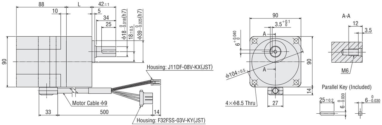
● Cable output in the opposite side of the output shaft
