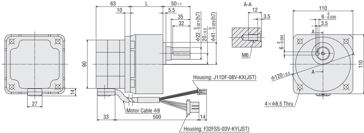
• Cable output in the opposite side of the output shaft
