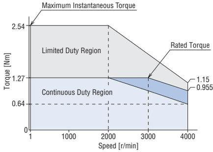
● The values correspond to each specification and characteristics of a stand-alone motor. The speed - torque characteristics show the values when rated voltage is applied.
