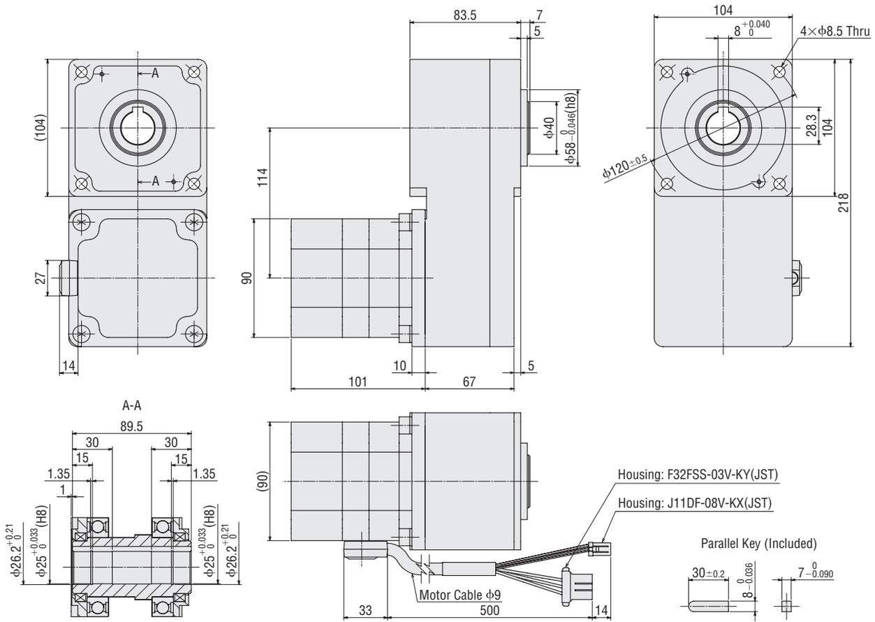
•Cable output in the opposite side of the output shaft
